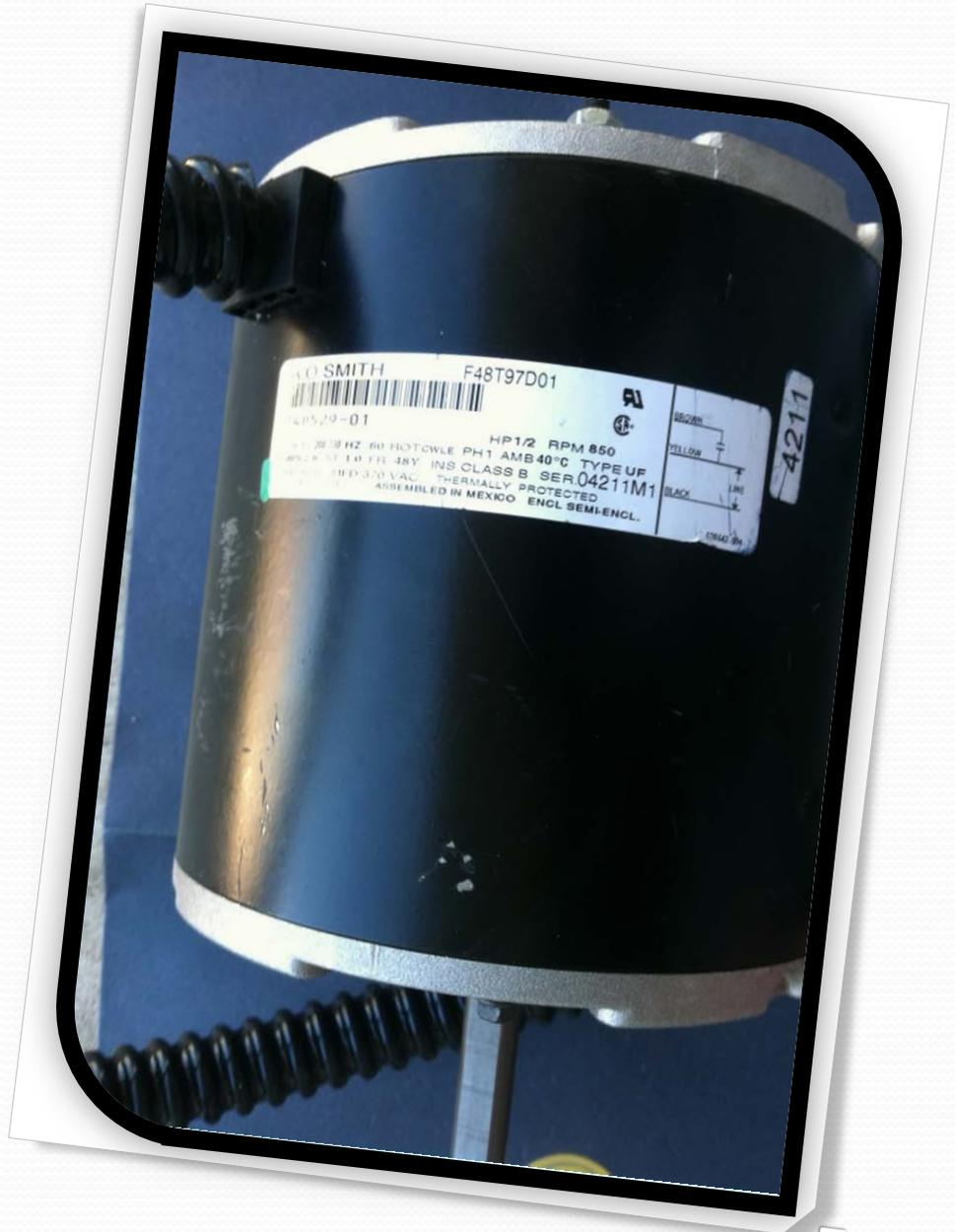
Next remove the black wire from the relay, the yellow and brown wires from the capacitor and the green wire from the back of the control box. The wires need to be pulled through the side control box, through the header plate and finally the plastic mould where the fan is located. (Next Page)
