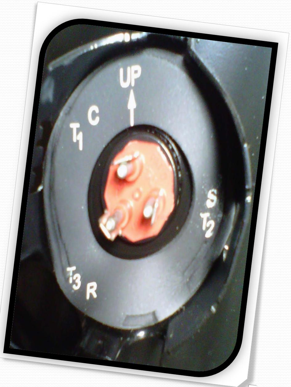
An additional indicator will be that the compressor will be very hot to the touch. The compressor will need time to cool down and the overload switch will have to close before the compressor will work. (you can not manually close the switch) If a test results in an open winding (OL) the compressor will not turn on.
