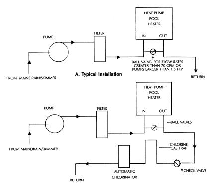
B. Installation with In-line Chlorinator
